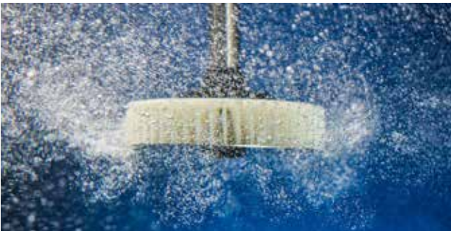
Turbine Aerator Head
